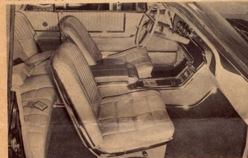
The unusual seats have moderately soft padding mounted in a complete metal shell. The result is outstandingly good.
